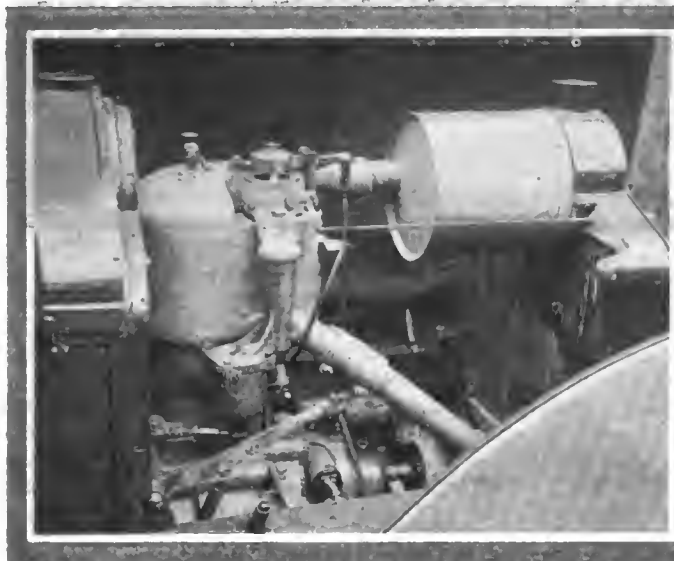
Carburetor Side of Sizaire One-Cylinder Engine
